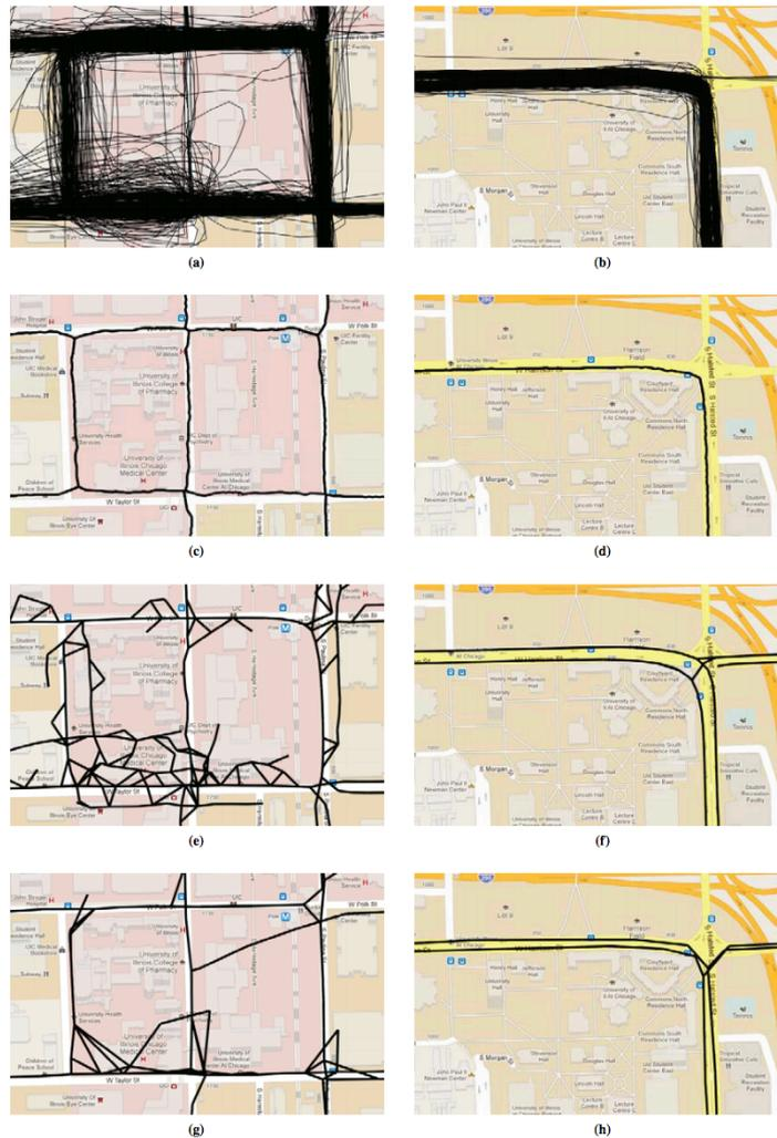
FIGURE 5 Raw data and results from three implemented algorithms in areas with high and low GPS error: (a) raw data, high-error sample; (b) raw data, low-error sample; (c) Davies algorithm, high-error sample; (d) Davies algorithm, low-error sample; (e) Cao algorithm, high-error sample; (f) Cao algorithm, low-error sample; (g) Edelkamp algorithm, high-error sample; and (h) Edelkamp algorithm, low-error sample.
